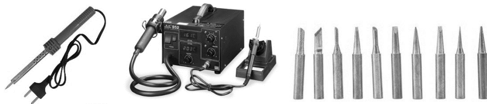
Gambar. Bentuk/Type Solder (solder ujung logam, Solder Blower, Ujung solder)
